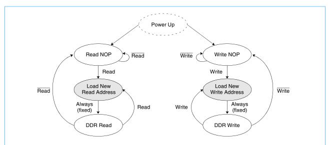
Notes: 1. Internal burst counter is fixed as two-bit linear; that is, when first address is A0+0, next internal burst address is A0+1.
